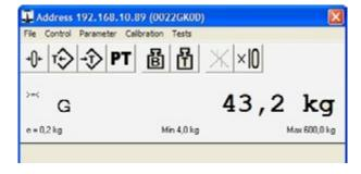
All parameter and calibration data are stored power failure safe in the instrument. The real-time clock runs at least 7 days without a power supply.
