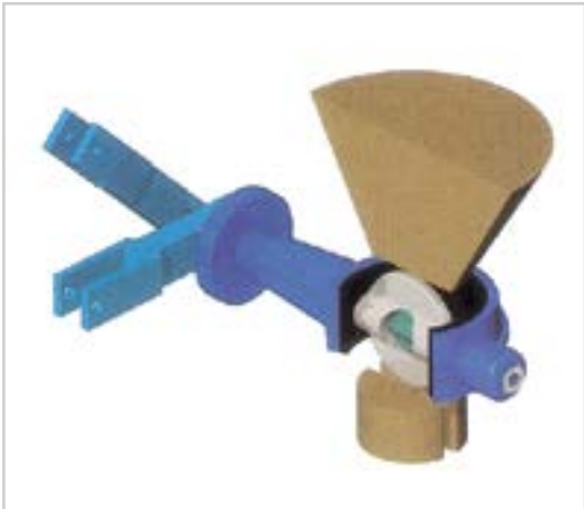
The main valve is opened for the coarse flow-through.
